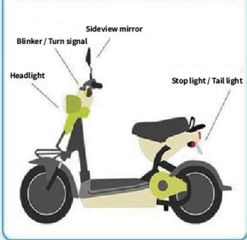
A motorbike should have the safety equipment of headlight, tail light, blinker, stop light and sideview mirror
